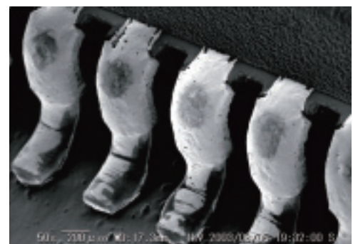
IC lead SnAgCu plating
